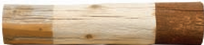
Media blasting. The bare wood shown in the middle DOES return to its natural color after media blasting.
